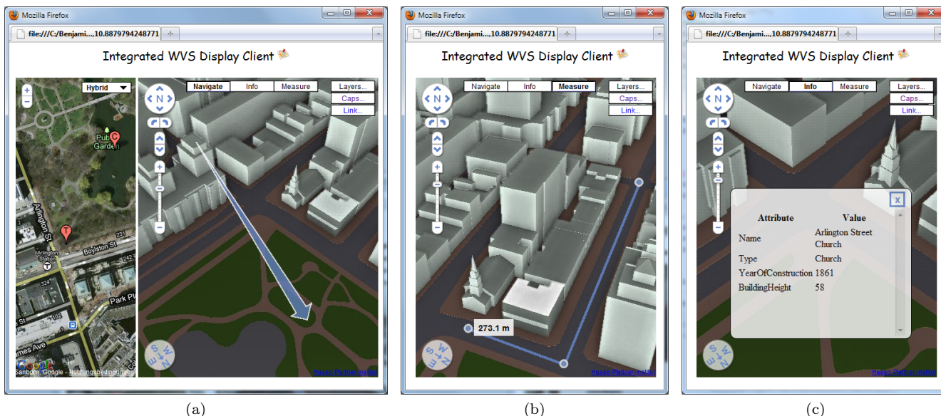
Figure 2.: Screenshot of a web-based WVS display client. (a) Integrated with a 2D map from Google maps, which marks camera look-to and look-from. The arrow indicates the selection of a new camera look-from and look-to within the image. (b) Specification of a path and display of its length. (c) Display of thematic information retrieved from the WVS for a feature selected by the user. (3D data: Boston Redev. Authority)
