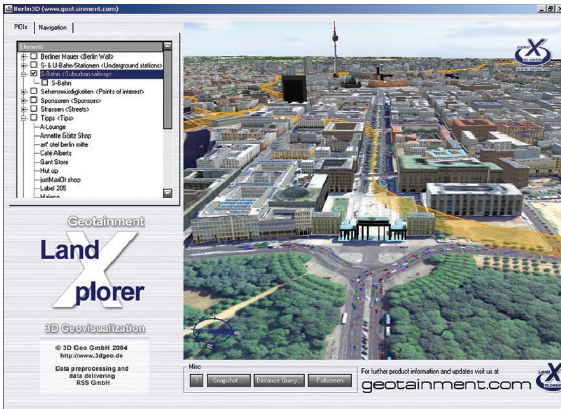
Figure 8 [below]. User interface of the interactive Berlin-3D application. Its implementation is based on the LandXplorer system and deploys constraints for both user guidance and DRM. The semi-transparent walls indicate the route of the underground railway system.
