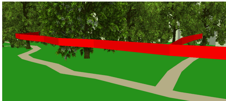
Fig. 3: Example for auxiliary objects representing potential eye positions of pedestrians walking along a park route.
