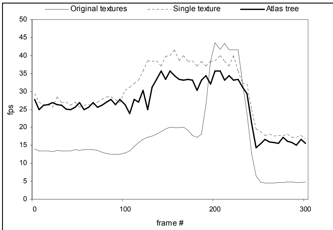
Figure 32: Frame rate comparison of different rendering configurations applied to the Chemnitz city model.
