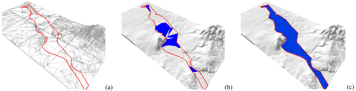
Figure 1. Vector data projected as polygons onto a level-of-detail terrain model, rendered in wire-frame style (a). Rendered with filled polygons: z-buffer artifacts are introduced since vector-data polygons tend to be coplanar with terrain polygons (b). Texture-based vector-data mapping does not produce artifacts (c).
