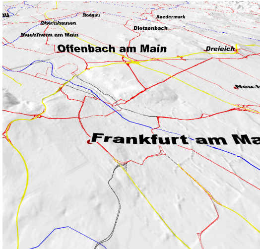
Figure 6. Hybrid representation of labels inside 2D texture and as 2D text objects. Far-away labels are displayed as billboards, they are not contained as elements of the terrain texture.
