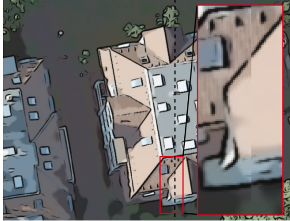
Fig. 5. A visible junction between two tiles in case a plain filtering is conducted. Edges are apparently interrupted and colors abruptly change
