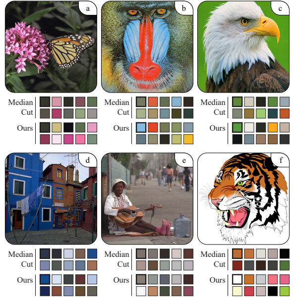
Figure 5: Comparison of the median-cut algorithm to our approach for dominant color extraction (the 10 dominant colors are sorted from left to right).
