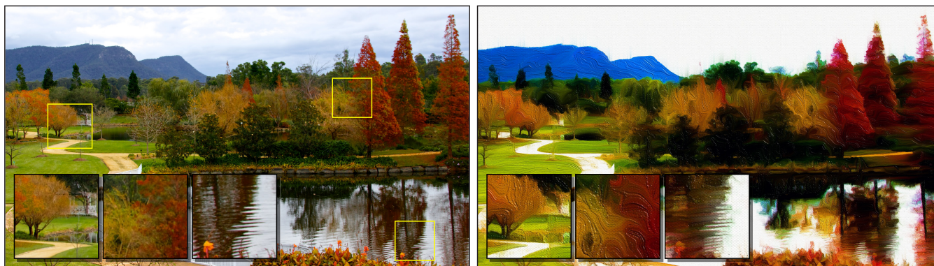
Figure 1: A result interactively produced with our mobile app for an input image with a resolution of 2,560 \times 1,800 pixels (left). The stylized output (right) is based on real-time color grading, multi-stage flow-based nonlinear filtering, and a paint texture synthesis.
