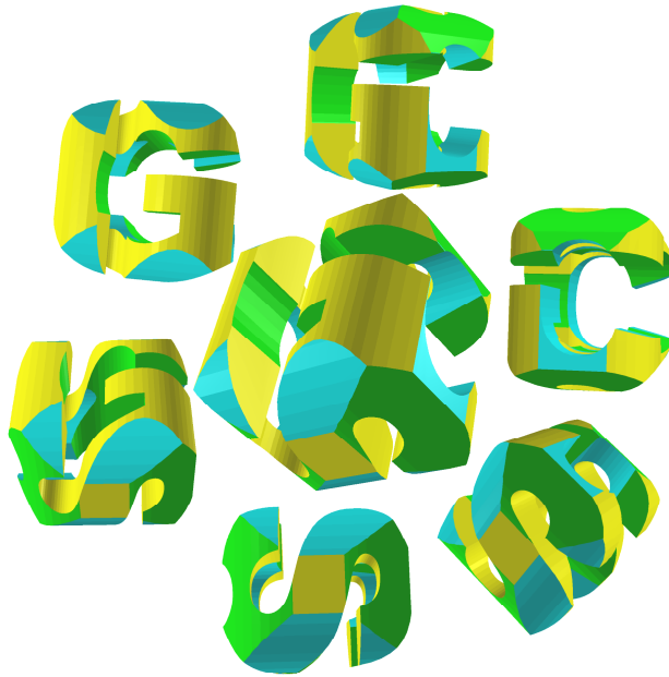
Figure 7. How does a 3D object look like that exactly fits through all letter-shaped holes? CSG gives the answer: Just intersect the extruded 3D-models of each letter. The resulting shape is shown below from different positions.
