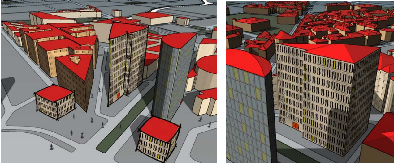
Figure 6: Real-time expressive virtual 3D city model based on stylized edges, enhanced edges, shadows, n-tone-shading, and procedural facade textures.
