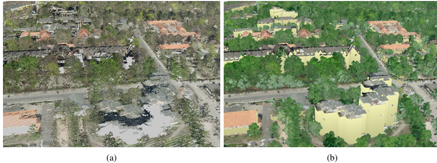
Fig. 1 (a) Example of a massive 3D point cloud rendered in a uniform way by GL_POINTS primitives and textured by aerial photography. (b) Same scene rendered by class-specific point-based techniques: different object classes can be better distinguished, holes on façades are filled, and visual clutter in the background is reduced.
