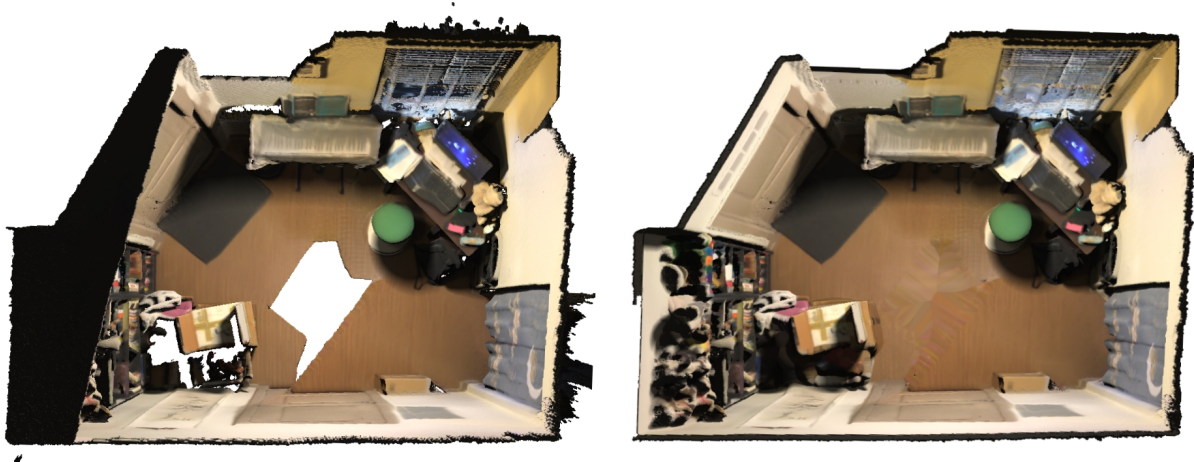
Figure 1: Signed Distance Function (SDF) reconstructed from ScanNet [Dai17] scan. Left image: Original SDF. The ceiling is shaded very dark as the virtual light source is located inside the room. Right image: Cleaned SDF using the implemented manipulation possibilities. The editing time amounted to 5 minutes.
