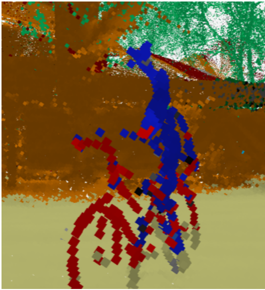
Fig. 7 Example of a composite classification (data by courtesy of Stadt Hamburg). Bicycle and cyclist are segregated by DL-based classification.
