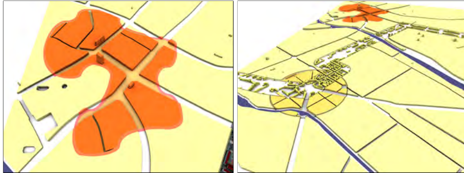
Figure 16: Generalization lenses allow the combination of different LOA representations in one image. Therefore, for example, focus regions of arbitrary shape (left) or the course of a buffered route, possibly overlapping other lenses (right), can be highlighted.
