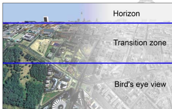
Fig. 4. Fixed image separation for the bird's eye view deformation
