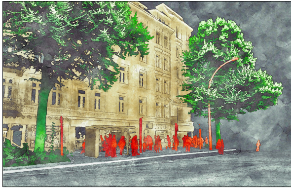
(b) Example result of a NPR of the same point cloud based on edge enhancement, class-specific coloring, ambient occlusion, and a watercolor postprocessing operation.
