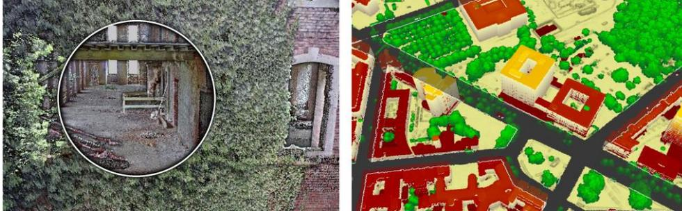
**Figure 6.** Focus+context visualization for massive point clouds. Left: Using an interactive see-through lens, the occluded interior of a building can be inspected in the context of the overall scan. Right: A visibility mask is used to highlight otherwise hidden street points.
