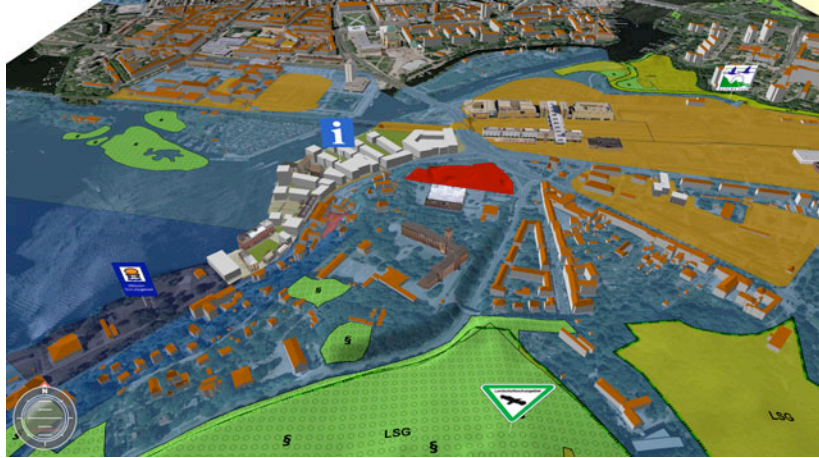
Fig. 6. Screenshot of the prototypic 3D Land Information System with integrated geodata including nature protection areas as raster-based terrain texture, water protection areas and polluted land cadastre as vector-based terrain textures.
