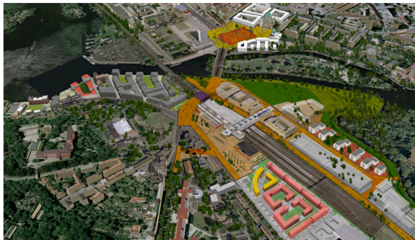
Fig. 5. Screenshot of the prototypic 3D Land Information System with integrated planning data (from top left clock-wise): 1. Master plan 'Speicherstadt' as extruded buildings and terrain texture; 2. Master plan 'Alter Markt' and development plan 'Landtagsneubau'; 3. Development plan 'Babelsberger Strasse' and construction plans for the residential building plots; and 4. Master plan 'Reichsbahnausbesserungswerk'.
