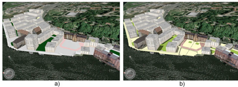
Fig. 8. The images show the results from the CityGML-based modelling approach for master plans; the left image shows the plan representation as a CityGML data set without a defined appearance for the land-use objects, while in the right image the plan graphics was used to texture the objects.
