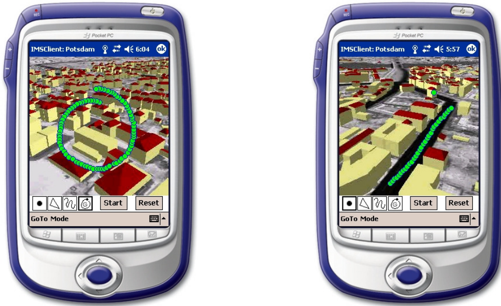
Fig. 1: Sketching the navigation command “look around” (left). Sketching the navigation command “walk along the path and, finally, look at the indicated building” (right).
