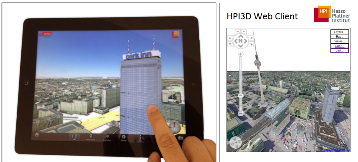
Figure 5: iPad application running the virtual 3D city model of Berlin using a WVS for image generation (left) and browser-based Javascript client supporting a stepwise interaction (right).
