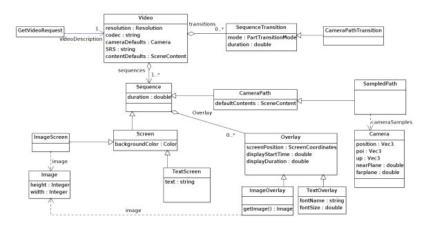
Figure 4: Excerpt of the object model for describing video presentations in a service request. A video contains one or more sequences, which may either be a camera path through a 3D scene or a screen (either an image or text). Two sequences are connected through sequence transitions that configure the blending properties and the interpolation between two adjacent camera paths.
