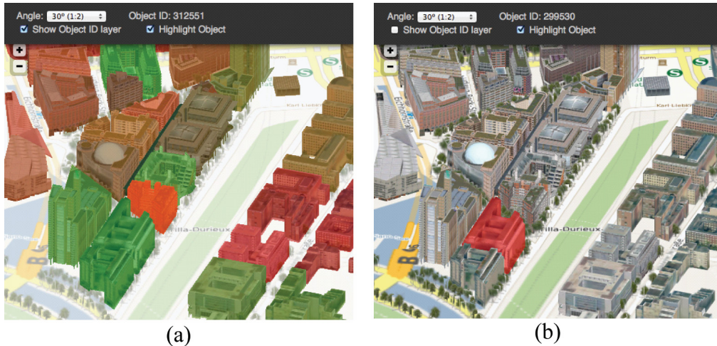
Figure 4. Example for client-side rendering effects implemented using a HTML5 canvas object id images. Subfigure (a) shows a debug view with object ids blended into the color image. Subfigure (b) shows the result of the highlighting effect for a specific object id.
