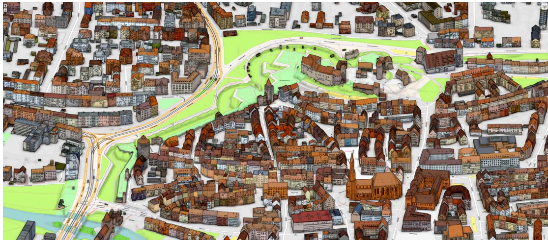
Figure 9.3: Web-based layered map showing the virtual 3D city model of Nuremberg with texture abstraction applied.
