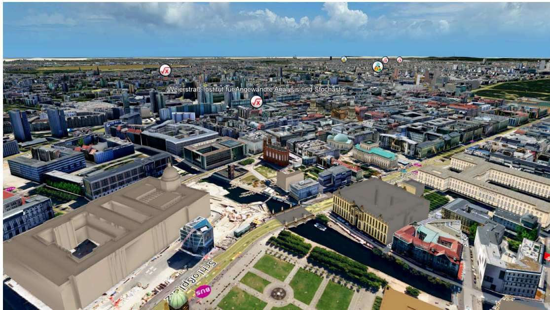
Figure 5.1: Example of an image generated by a GetView request. It shows the virtual 3D city model of Berlin, layered terrain textures (road names on top of the aerial image), planning models (palace at the bottom left in shaded style), POI layers with labels. Several rendering effects are applied as image styling (screen space ambient occlusion, anti-aliasing, color improvement).
