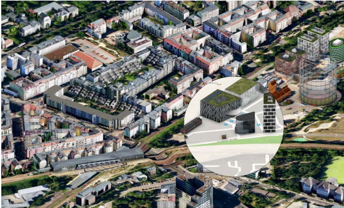
Figure 6.4: Example of a web-based layered map using an information lens to combine two map layers in one view. The context layer shows the textured virtual 3D city model and an orthophoto as terrain texture. The focus map is configured to show a different configuration, i.e., a planning model and a street map as terrain texture.
