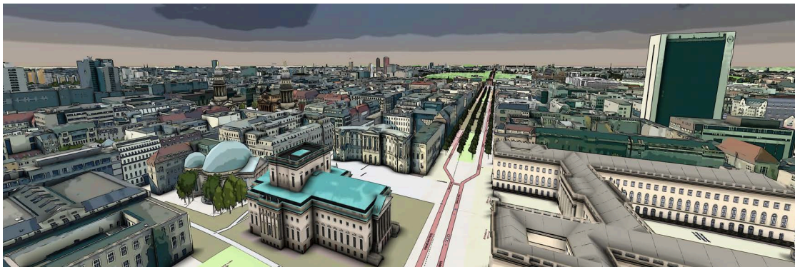
Figure 5.9: An example of image-based styling applying multiple image styles (a non-photorealistic rendering style combined with screen-space directional occlusion) being applied on a view of the virtual 3D city model of Berlin. Although there is a large number of features portrayed in the image, the execution time for the rendering effect remains in an equal range since execution times only depend on image resolution instead of number of features portrayed.
