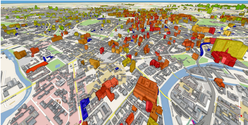
Figure 5.7: Example of thematic styling: Visualization of available apartments and their pricing based on the Berlin virtual 3D city model. The 3D rendering service applies styling for each of the 600,000 building models using two visual variables: 1) Buildings that are out of scope (no apartments available) are flattened and the building textures are desaturated. 2) Buildings of interest are scaled up and their textures are blended with colors reflecting the rental price per square meter.
