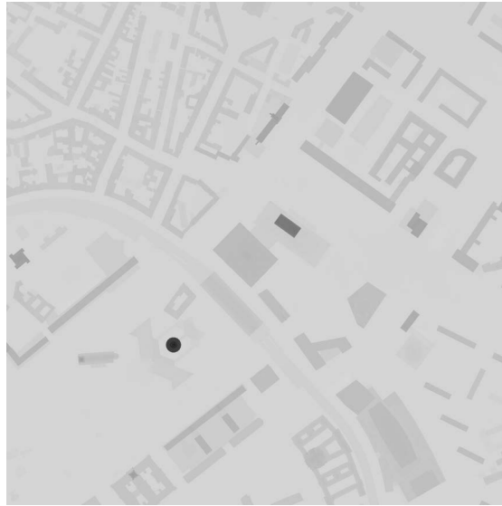
Figure 8.3: Example of a depth map covering 1\text{km}^2 around the Alexanderplatz in Berlin. The image was generated by a 3DPS from the virtual 3D city model of Berlin. It contains gray values encoding the normalized distance from camera near (black) to far plane (white).
