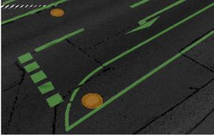
Figure 3. Point clouds with detected manhole covers (orange) and road markings (green) represented as shapes rendered on top of the point cloud.
