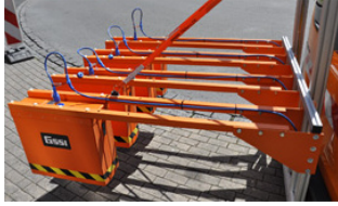
Figure 7. Ground penetrating radar antennas mounted to the measuring vehicle.
