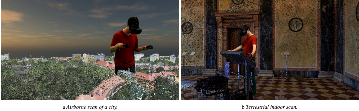
Figure 1: Examples of massive 3D point clouds being immersively visualized using our rendering system and an HTC Vive. Supported interaction techniques include measuring of distances as well as rotating and scaling of the rendered data.
