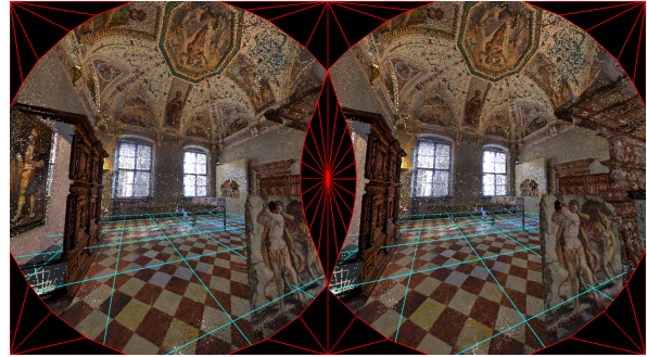
Figure 5: A separately rendered mesh serves as a mask to discard fragments beyond the visible area of an VR device’s screens early on.
