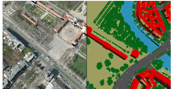
Figure 3: Different color schemes can be applied at runtime. Left: RGB colors extracted from aerial imagery. Right: Colorization based on surface categories.
