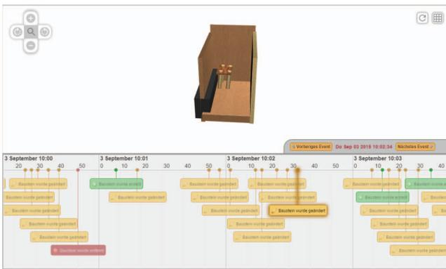
Figure 4. The Tele-Board Prototyper history browser. Users can navigate to any point in time of a prototype's course of development using the timeline. A branch of a prototype can be created at a specific state in order to follow a different development path.
