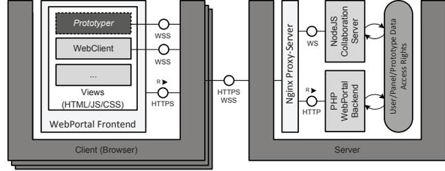
Figure 3. The Tele-Board client-server architecture. Web portal and 3D model synchronization is managed by an Nginx proxy server using a single standard port 443 for encrypted communication.
