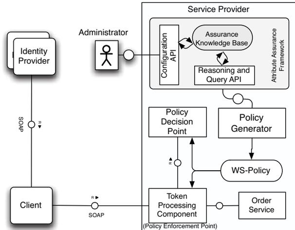
Figure 4. Architecture of the service provider using the Attribute Assurance Framework.
