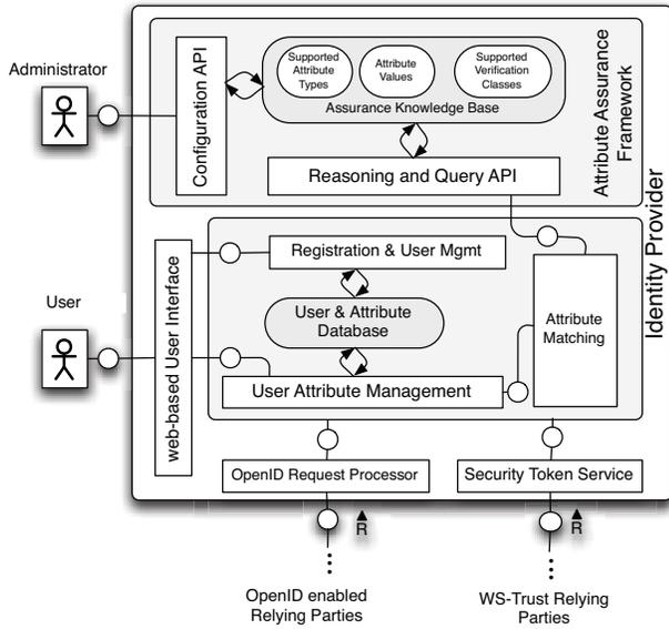
Figure 2. Architecture of our identity provider using the Attribute Assurance Framework.
