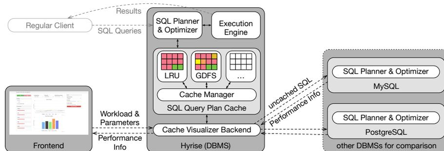
Fig. 2: Architecture of the Cache Visualizer.
