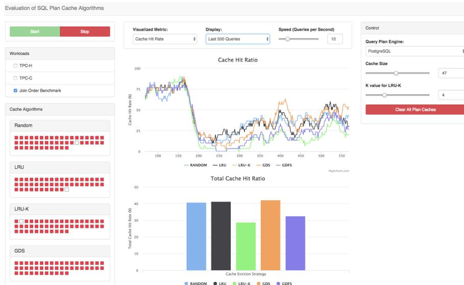
Fig. 1: Screenshot of the Cache Visualizer. The left side shows the different caches. Red blocks symbolize currently cached items. White blocks show which items are evicted. The main graph shows the performance of different compared cache algorithms. Parameters can be chosen on the right.
