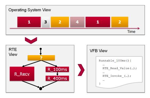
Fig. 5. Relationship between Operating System, Runtime Environment and Virtual Function Bus with respect to the integration of runnables
