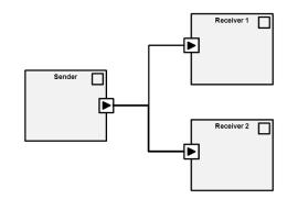
Fig. 7. VFB Model for a sender-receiver communication topology
