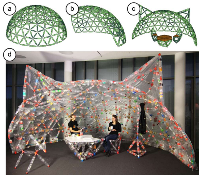
Figure 13: (a) Dome created using the dome tool. (b) We make the opening using the delete tool, and (c) add decoration using the triangle and line tools. (d) The resulting dome is built using 512 bottles.
