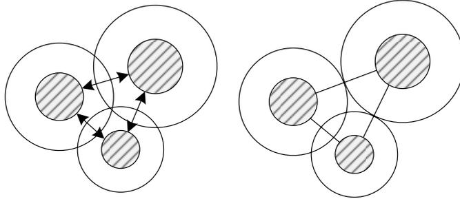
**Fig. 5:** Spring model for mutual landmark displacement. It shows original landmark positions before (left) and after (right) the application the model spring.
