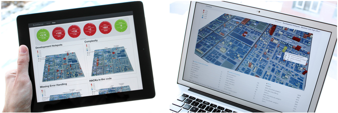
Figure 1: Left: Dashboard accessed from a tablet computer, which summarizes project specific performance indicators (metrics) and links them to software maps. Right: Software map with code metrics mapped to ground area, height, and color, rendered in real-time in the browser.
