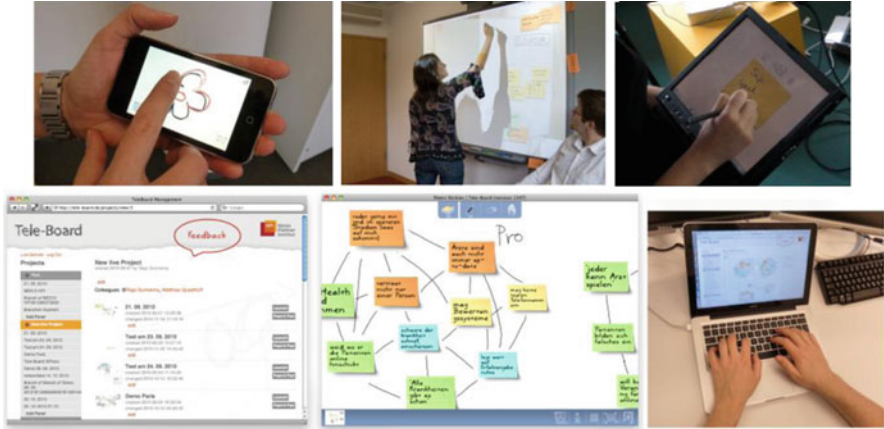
Fig. 3 Tele-Board and its components (from top-left to bottom-right): StickyPad on iPod touch, whiteboard interaction, StickyPad on tablet PC, web application, screenshot of the whiteboard client, editing with a laptop computer
