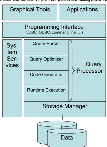
Figure 1: A generic DBMS architecture
