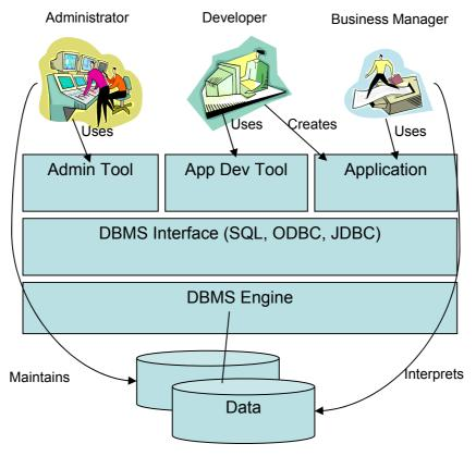
Figure 2: Three Roles for DBMS Usage
