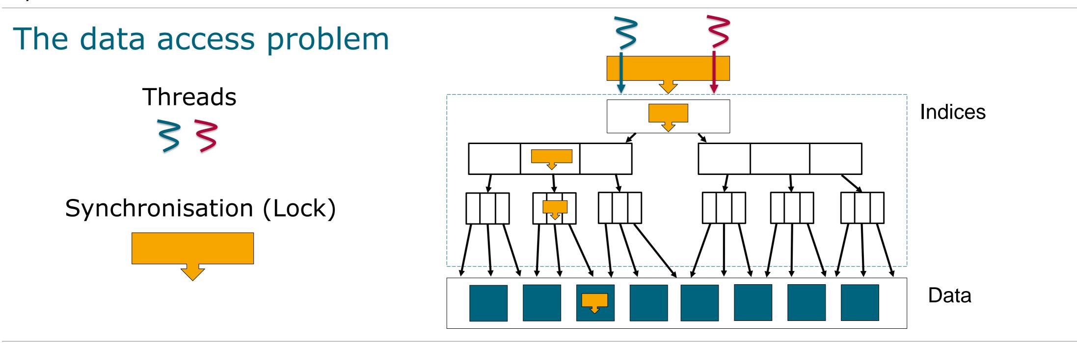
Physiological partitioning (PLP) describes the process where the index of the same address space is split into different ranges. Those ranges get assigned to specific threads. As you can the in the following example the indices of the data got separated into two ranges and get assigned to different threads. This means that those two threads should rarely wait on the other thread for data access because they only access separate sections of the indices.
