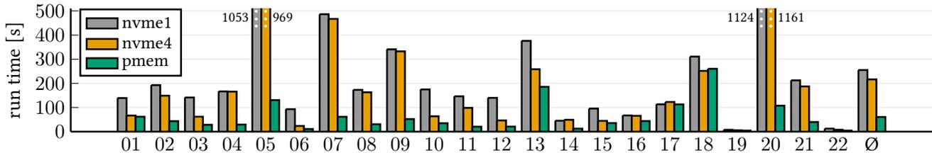
Figure 6: TPC-H results (scale factor 100) on Postgres running on a single NVMe, a RAID 0 of four NVMe, and PMem.
