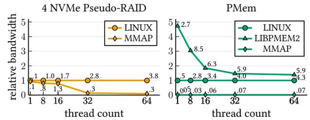
Figure 4: Relative bandwidth of `mmap+msync` and `libpmem2` to Linux I/O for the buffer management workload, for 4 KiB pages and 80% writes. Note that the plot shows relative performance, and absolute performance numbers in GiB/s for each data point are given.
