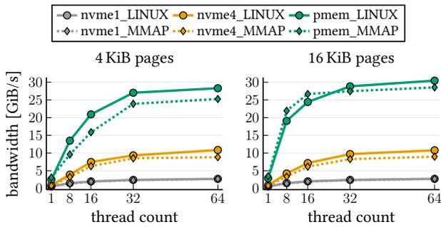
Figure 2: Bandwidth for the table scan workload.
