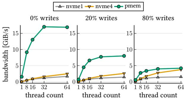
Figure 3: Bandwidth for the buffer management workload with 4 KiB pages.
