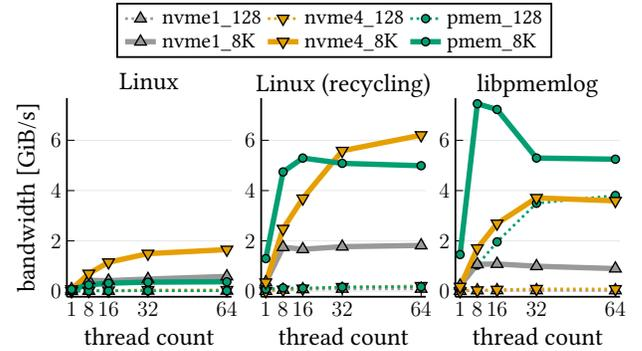
Figure 5: Bandwidth for the logging workload.
