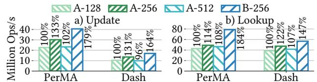
**Figure 10: Hash index in PerMA and Dash. 16 threads. PerMA: 512 Byte lookup + 2 64 Byte Cache update. Dash: 8/8 Byte key/value.**
