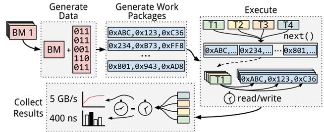
Figure 3: Execution cycle of a benchmark in PerMA-Bench.
