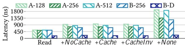
Figure 7: 256 Byte random read + write latency. 16 Threads.
