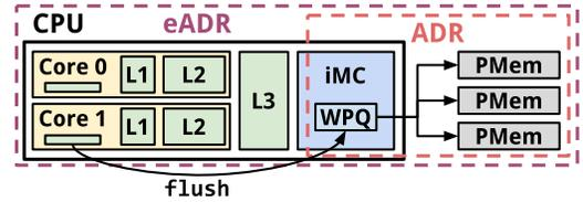
Figure 2: Writing to NVDIMM-Ps from the CPU.
