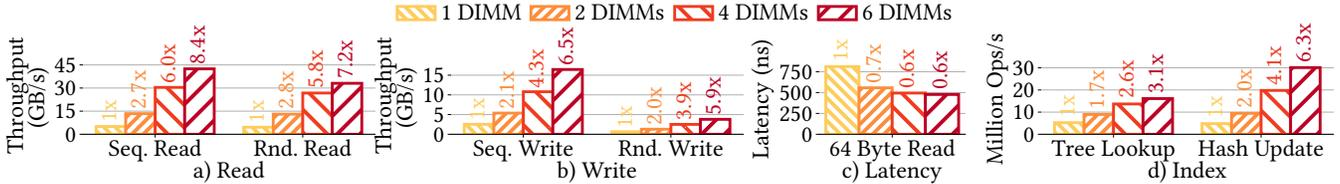
**Figure 15: Impact of number of DIMMs in the server (Apache-256).** All runs with 16 threads. Sequential/random reads with 4096/256 Byte access size. Sequential/random writes with 512/64 Byte access size and *NoCache*. Tree with 512 Byte nodes. Hash with 256 Byte buckets.
