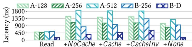
Figure 8: Double-flush latency. 64 Byte read + 2 64 Byte write.
