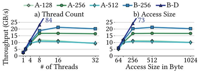
**Figure 5: Thread and access size impact on sequential writes.**
