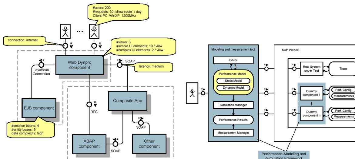
The left figure shows how a sample scenario in this project could look like. Additionally to the depicted static structure a sequence chart is necessary for running the simulation. The right picture shows the existing modeling and simulation framework, which will be extended during this project.
