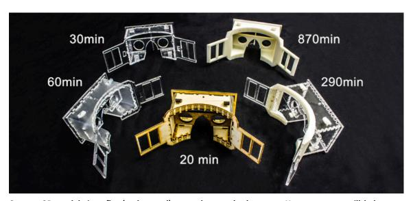
Convert 3D models into flat (and curved) parts that can be laser cut. Your converter will help users fabricate this head-mounted display, for example, by a factor of up to 40x.
