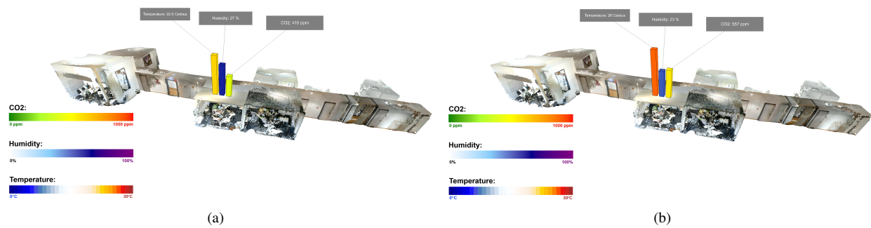
Figure 6. Visualization of combined room temperature, humidity and carbon dioxide captured for two time points: (a) t_0 : 22.6 Celsius, 27 % and 415 ppm. (b) t_1 : 26 Celsius, 23 % and 557 ppm.
