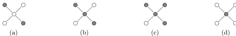
Figure 3: Different cases of crossing edges. (a) Intersection of a passable and an unreachable edge. The dummy vertex (center) is reachable. The unreachable edge is split into two boundary edges. (b) Intersection of an accessible and an unreachable edge. The dummy vertex is unreachable, dashed edges indicate new boundary edges. (c) Intersection of an unreachable edge and a boundary edge, creating unreachable edges and a new boundary edge. (d) An intersection of accessible edges creates an unreachable vertex and four boundary edges.
