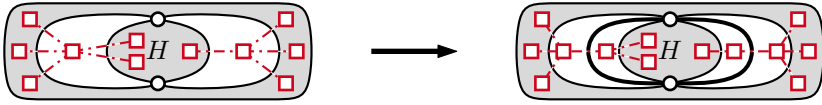
Fig. 2. Adding the safety edges (bold) to G and the effects on the dual graph
