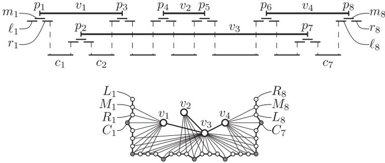
Fig. 14. An example graph  $H$  containing the vertices  $v_1, \dots, v_4$  with prescribed interval representation  $I$  together with the markers  $\ell_i, m_i, r_i$  and the connectors  $c_i$  on the top. The resulting graph  $G'$  with the new vertices  $L_i, M_i, R_i$ , and  $C_i$  on the bottom.
