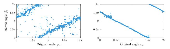
Fig. 6. The plots correspond to embeddings with average squared deviation  $\Delta \varphi_G = 0.44$  (left) and  $\Delta \varphi_G = 0.01$  (right). For each vertex v the plot contains one point with x-coordinate  $\varphi_v$  (angle of v in the original embedding) and y-coordinate  $\widehat{\varphi_v}$  (angle in the computed embedding). The embedding is considered good if the plot resembles the identity function f(x) = x up to cyclic shift and rotation.
