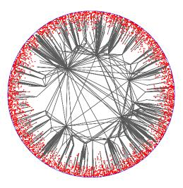
Fig. 9. When the average degree  $\delta$  is small for the graph generation, most nodes (shown in red) are not part of the giant. It becomes hard to infer the original number of nodes based on the few that remain in the giant component.
