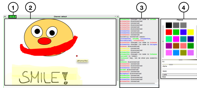
Figure 50: User interface of the SyncMorph with (1) buttons to toggle and indicate connection state, chat pane and pencilstyler (2) synchronization pane, (3) chat pane and (4) pencil styler
