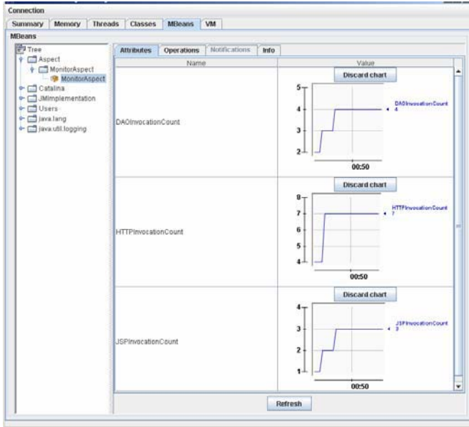
Figure 7. Data from aspects is visualized and can be updated in JConsole.
