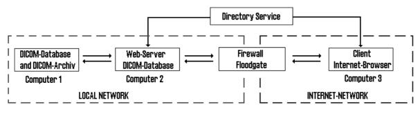
Figure 1 Structure of the internet/intranet information system for the transfer of DICOM data
