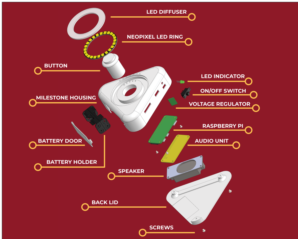
Figure 5.6: Milestone exploded view
