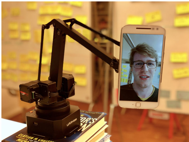
Figure 3.40: Our prototype with a smartphone being mounted to a movable robot arm. The Arm automatically turns the smartphone to reflect where a human would pay attention to.
