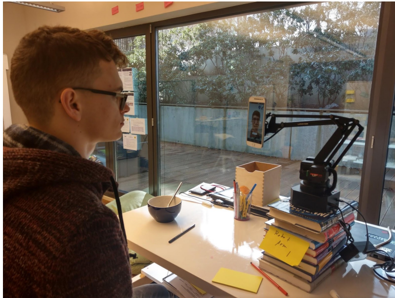
Figure 3.41: The robot arm on which the phone is mounted automatically moves it, so the caller can see the user who is talking.
