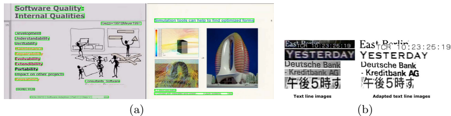
Fig. 3. (a) Text detection results. All detected text regions are identified by bounding boxes. (b) Text binarization results of our dynamic contrast-brightness adaption method.
